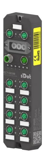
P67 I/O module, supporting various bus protocols. The product size is 225\*62\*35, and the shell is made of PTB+GF30% reinforced plastic material, which has excellent mechanical properties; the fully sealed design can be used in harsh working environments. There is a wide variety of signals available, providing a diverse range of options for on-site applications.
