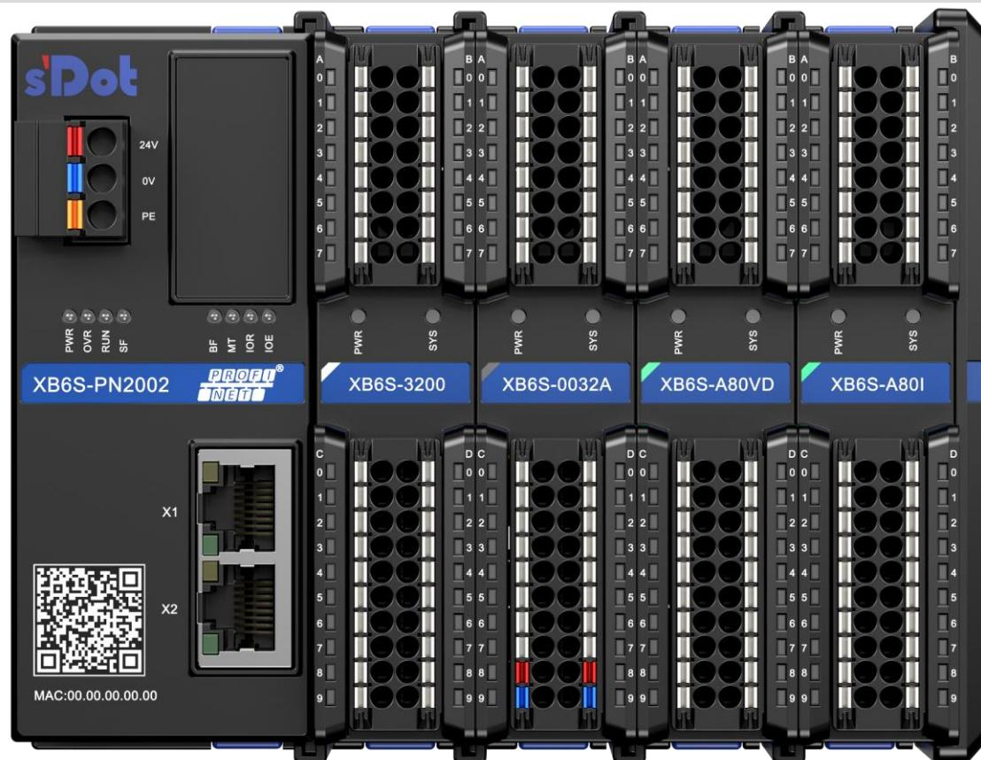
**产品组合方式二 (耦合器模块、I/O 模块、扩展电源模块、I/O 模块、终端盖板)**
