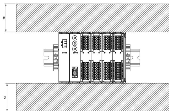
**确保模块竖直安装**
