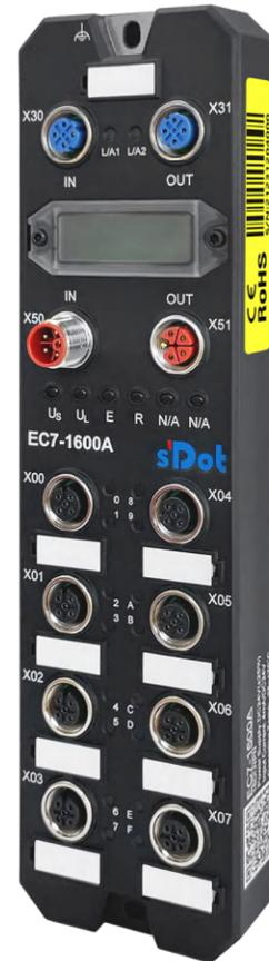
Solidot IP67 I/O modules support various bus protocols. The size of the product is 225\*62\*35mm. The shell is made of PTB+GF30% reinforced plastic material with excellent mechanical performance. The fully sealed design is suitable for harsh working conditions. A wide range of signal types provide diverse options for field applications.
