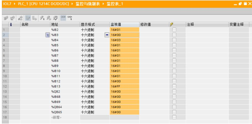
The screenshot shows a monitoring table for PLC\_1 [CPU 1214C DC/DC/DC]. The table has columns for Name, Address, Display Format, Watch Value, Modify Value, and Notes. Rows 1 through 17 show various addresses like %IB2, %IB3, etc., with their respective values and formats. Row 17 is highlighted with a yellow background. Row 18 is a new entry row labeled '<新增>'.
