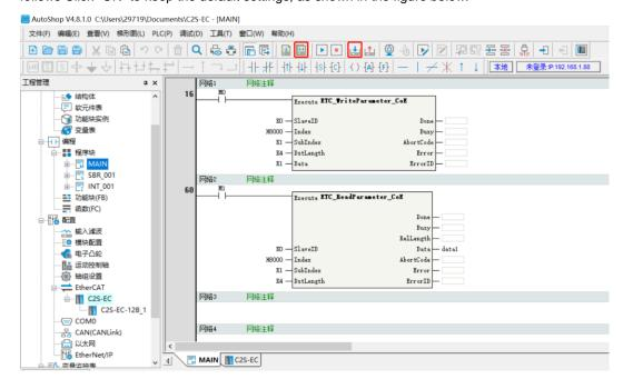
k. After the download is complete, click the "Run" button on the toolbar, and then click the "Monitor" button on the toolbar, as shown in the figure below:
