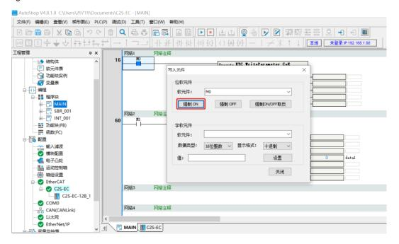
n. Similarly, right-click on M1 under Network 2 on the MAIN page, select "Write" to bring up the Write Component window, and then click "Forced ON" to execute the read command, as shown in the figure below:
