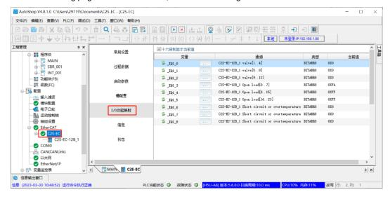
b. Double-click the button to the right of the first group of channels IQ1-0, the pop-up window to write components, enter "255", click "Set" to open the first group of solenoid valve coil channels, as shown in the figure below:
