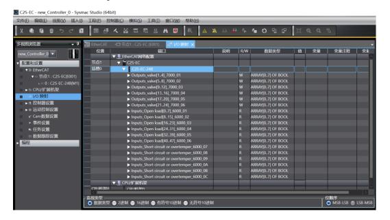
b.Outputs\_valve[1...4]~Outputs\_valve[21...24] has a total of 6 groups and 48 channels solenoid valve coils with control function. Select the corresponding channel, you can control the solenoid valve coil through the modification of the channel value. If the value is "TRUE", it means open and if the value is "FALSE", it means close, as shown in the figure below.
