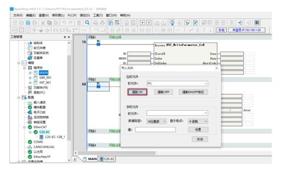
o. After the read is completed, you can see that the Data value in the read instruction changes to 1, i.e., the 8000:01 clear/hold parameter is set to 1 hold, as shown in the figure below:
