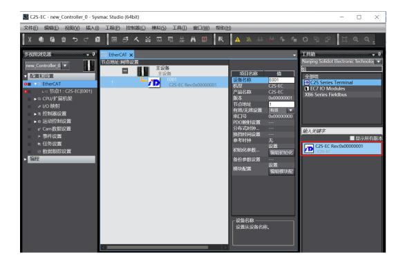
c. In the EtherCAT main page, click to select "C2S-EC", and then click "Edit Module Configuration" in the right menu, as shown in the figure below:
