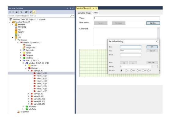
If you want to control the output of a group of solenoid valve coils, take the first group of channels as an example, you can click "valve[1...4]" under "Outputs" in the left navigation tree, click "Write" in the corresponding "Online", enter the value "255" in the corresponding "Dec" in the dialog box, and then click "OK". Then you can open the first group of solenoid valve coil channels, as shown in the figure below:
