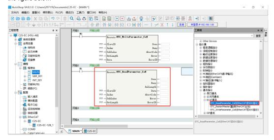
g. According to the startup parameter in step a, you can know the information of the parameter's Index, SubIndex and DataLength, etc., and fill the information into the write and read instructions. For example, 8000:01 clear/hold parameter, IndexIndex is 8000, SubIndex is 1, BitLength is 32 i.e. 4 bytes, DstLength is 4, write it into the item on the left side of the read/write instruction and SlavECD is written to 0, as shown in the figure below:
