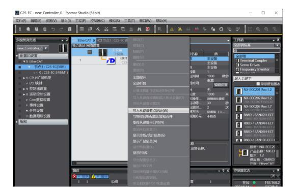
c. In the Set Node Address window, click the value under Set Value, enter the node address, and click the Write button to change the slave device node address, as shown in the figure below:
