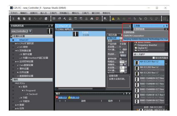
b. Click "C2S Series Terminal" to select the product series, select the product model at the bottom, and double-click "C2S-EC" to add the slave device, as shown in the figure below:
