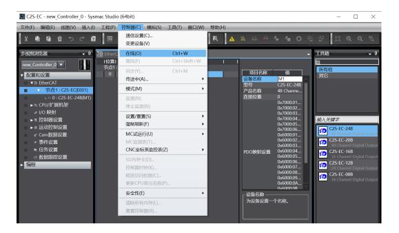
b. Right-click on the master device, click and select "Write Slave Device Node Address" as shown in the figure below:
