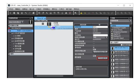
d. In the main page of module configuration, click to check the position of slot 0, and then in the right side of the toolbox, you can see the module model number "C2S-EC-24B", double-click to add the module to the slot, as shown in the following figure. Add all modules one by one according to the actual installation topology.
