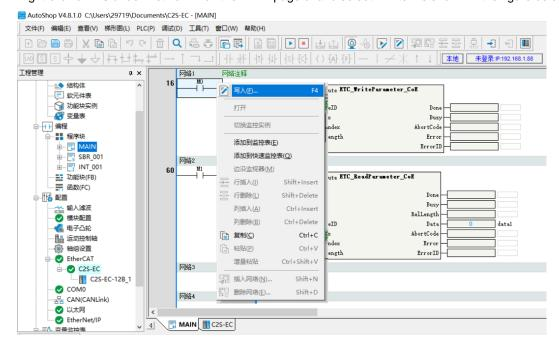
m. The Write Component window pops up, click "Force ON" to execute the write command, as shown in the figure below:
