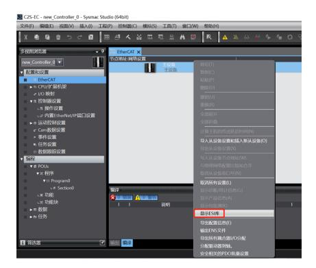
b. In the pop-up "ESI Library" window, click "Install (file)" button, select the XML file path, click the button "Yes" to complete the installation, as shown in the figure below:
