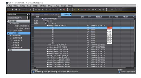
c. Inputs\_Open load[0..7]~Inputs\_Open load[40..47] has a total of 6 groups and 48 channels solenoid valve coils with control function. You can select the corresponding channel to view the diagnostic value (the diagnostic value is valid when solenoid valve coils is off). If the value is "TRUE", it means open circuit. If the value is "FALSE", it means normal status, as shown in the figure below:
