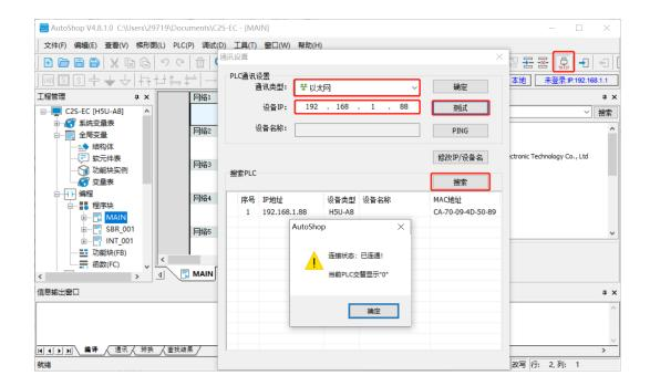
b. If the communication test fails, check the IP address of the computer, which needs to be in the same network segment as the IP address of the PLC device. Modify it and test again.
