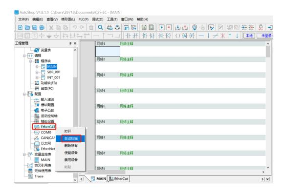
b. The automatic scanning window pops up, click "Start Scanning", after scanning the device, select the device, click "Update Configuration", as shown in the figure below:
