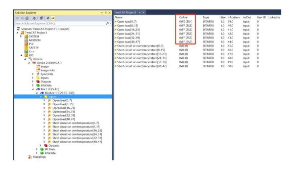
Expand a set of Open loads in the left navigation tree and click on any channel to view the open diagnostic value of the solenoid valve. For example, click the folding symbol to expand Open load[0..7], click Open
