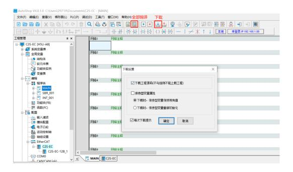
b. After the download is completed, click the "Run" button on the toolbar, and then click the "Monitor" button on the toolbar, you can see the successful configuration in the left navigation tree, as shown in the figure below:
