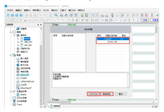
c. After the configuration update is completed, the added devices can be seen in the left navigation tree as shown below:
