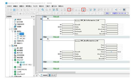
I. Right-click on M0 under Network 1 on the MAIN page of and select "Write". is shown in the figure below:
