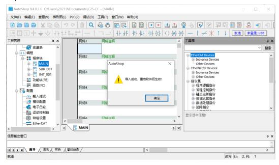
d. Import the previously created project, you can view the imported files in the right toolbox, as shown in the figure below:
