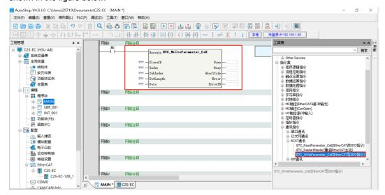
e. Click the area below the MAIN page network 2, click the toolbar Normally Open Contacts button, pop-up window of the normally open contacts, select the number of 1, click "OK", as shown in the figure below:
