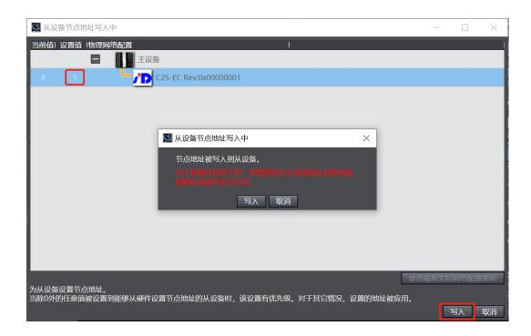
d. Power down and reboot the slave device when prompted after the node address is successfully written.
