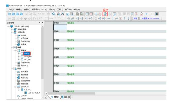
c. Click the area below Network 1 on the MAIN page, click the Normally Open Contacts button in the toolbar to bring up the Normally Open Contacts window, select 0 for the number, and click OK, as shown in the figure below:
