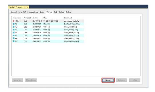
b. In the "Edit CANopen Startup Entry" interface, you can see the setting parameters 8000:0 and 8200:0. After expanding the parameters, 8000:0 is the function of setting parameters for all channels uniformly, and 8200:0 is the function of setting parameters for a single channel or a group of channels, as shown in the figure below:
