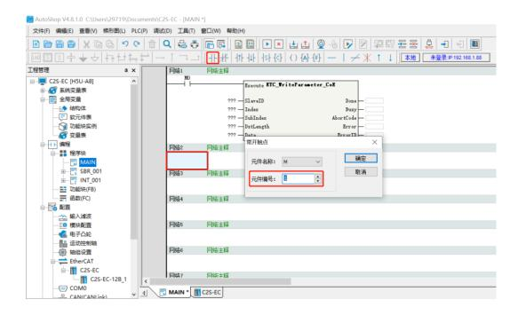
f. Double-click "Command Set -> Communication Commands -> ECAT Communication -> EtherCAT Read SDO Command" in the toolbox on the right to add the read command to the MAIN program, as shown in the figure below:
