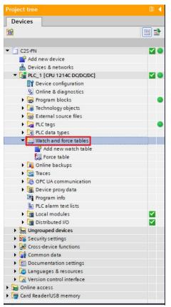
b. Double-click "Add New Monitoring Table" and the system will add a new monitoring table, as shown in the figure below.
