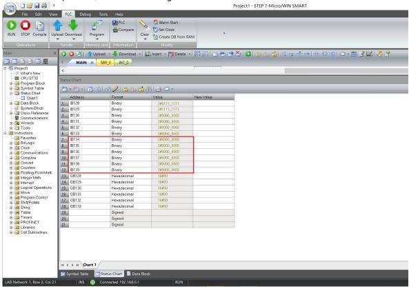
e.Channel **output control**, if you want any group of solenoid valve coil outputs in the valve terminal to turn on, taking the first group of channels as an example, you can enter "16#FF" in the "New Value" cell of QB128 and click the write button, you can open the first group of solenoid valve coil channels, and other channels open the output method 1 To, as shown below.
