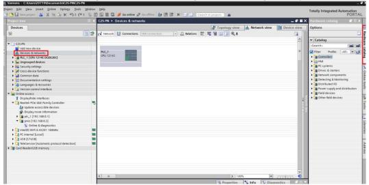
c. Find the "C2S-PN-24B" module in the hardware directory, drag or double-click "C2S-PN-24B" to " Network View", As shown below. If you want to connect multiple modules, you can connect them under the "Hardware Catalog" on the right., add modules in sequence according to the actual topology.
