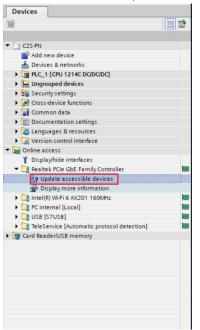
b. After the update is completed, the connected slave devices are displayed, as shown in the figure below.
